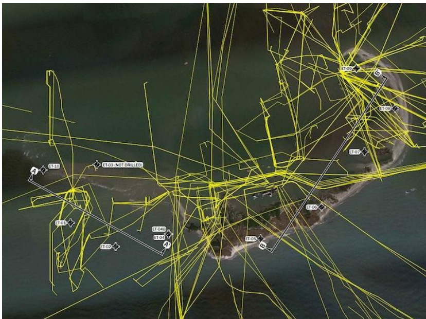
Figure 4. Oil and gas pipelines in, under and around East Timbalier Island, Louisiana. 7
