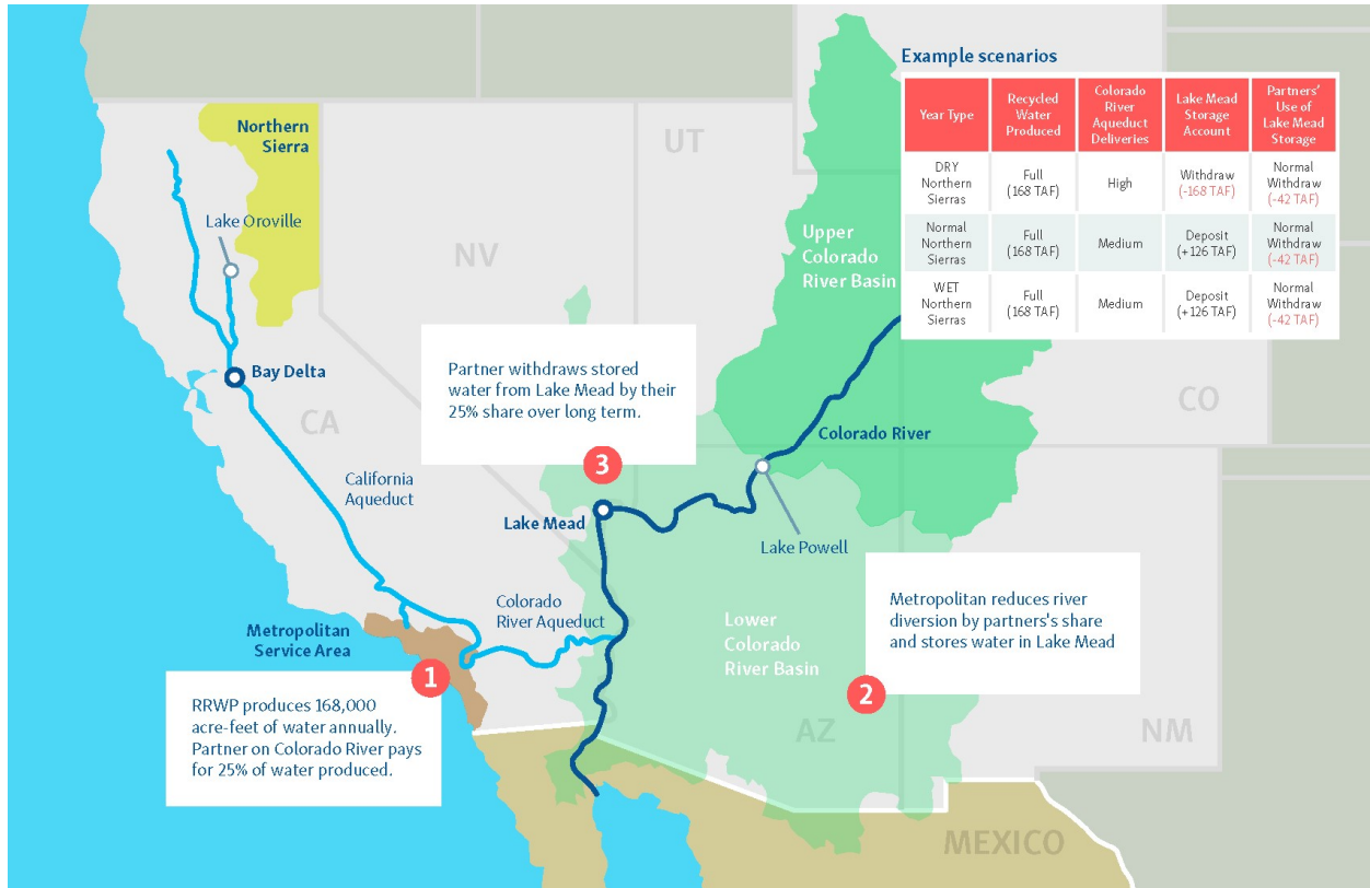
Figure 2. Metropolitan's Conveyance System and the Regional Recycled Water Program Connect Two Critical Watersheds
